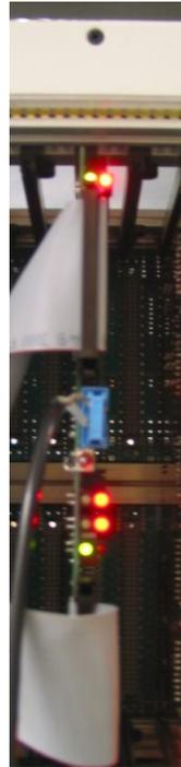
The top set of 2 LED's are on the top of the passth4 card. The bottom set of 6 LED's are just below the toggle switch (which in photo is just below blue).
