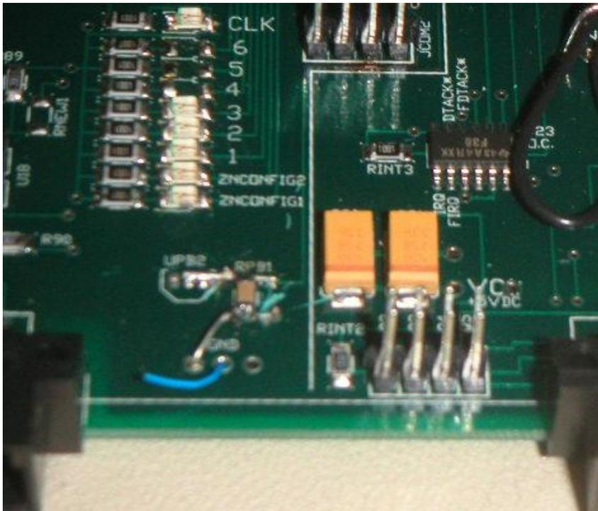
On PASSTH4, these connections must be made by hand. (See Steve, who will solder on a small wire onto the connector, a simple “jumper” to allow cards to the right to receive signals.
