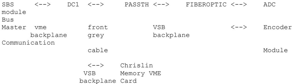
Set up commands come from the user's computer via the SBS VME master, and are passed in a standard manner, over the VME backplane to the commercially supplied DC1 card (from Access Dynamics 505 345 7637). This
