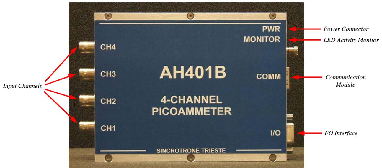
Fig. 1 - The AH401B I/O Connections
